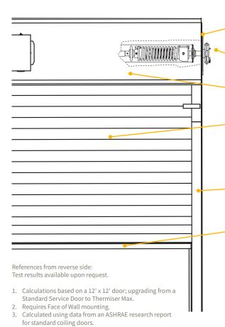
**BRACKETS** - Powder-coated steel brackets match the curtain, bolting to the guide assembly to support the counterbalance shaft and curtain.
