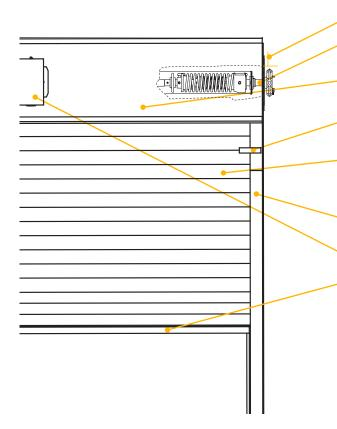
**BRACKETS** - 304 stainless steel with a zinc plated flange bearing.
