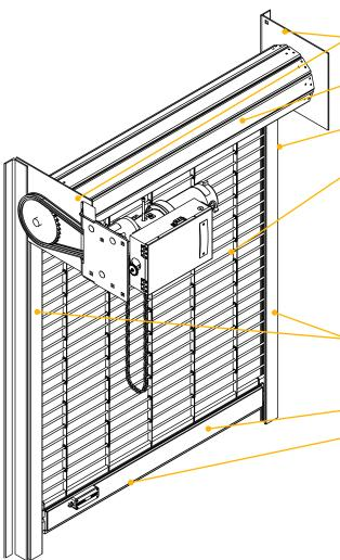
**BRACKETS** - Steel with SpectraShield® powder coating in Gray. Bolt to guide assembly and support counter-balance shaft and curtain.
